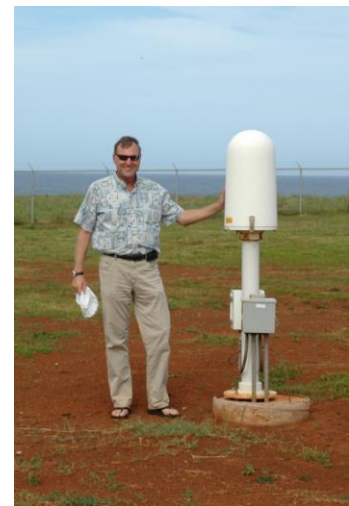
Dr. Businger with a long-range, lightning sensor (manufactured by Vaisala) located at Lihue airport in Kauai, Hawaii. The lightning sensor works 24 hours a day, 365 days a year to detect electromagnetic signals produced by lightning. Photo credit: Businger
